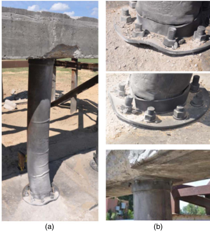
Fig. 9. Deformation of MSJC after blast test: (a) global; (b) local [(a and b) images by Michel Bruneau]
