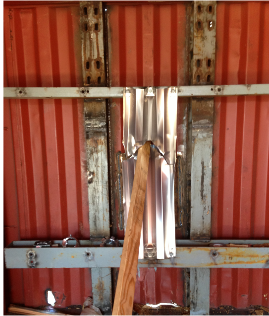
Figure 24: Panel Failure at KE_m = 1.500\text{kJ}
