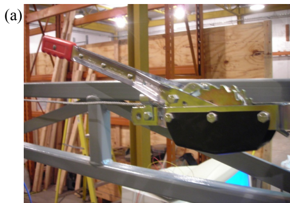
Figure 9: Horizontal mobility components of the LSU wind cannon: (a) hand winch, and (b) pulley system
