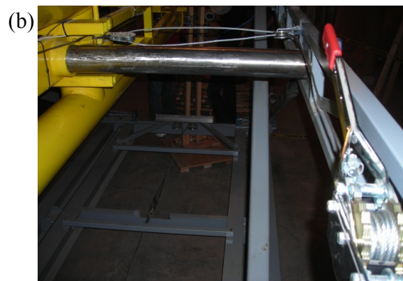
Figure 9: Horizontal mobility components of the LSU wind cannon: (a) hand winch, and (b) pulley system
